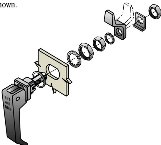
3. Pawl should be adjusted to GRIP measurement with the door open and the handle in the LATCHED position. Use two wrenches to tighten.
