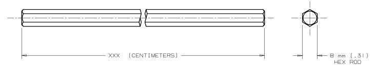
THE THREE DIGIT NUMBER IN THE PART NUMBER IS THE OVERALL LENGTH IN CENTIMETERS
