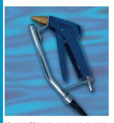
Model 4100 is a heavy duty ionised airgun for removing dust and other contaminants from sheets, mouldings, optics, electronic assemblies, automobile bodies and extrusions. It kills the static charge on both the dust and the substrate to allow a thorough cleaning.
