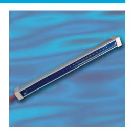
Model range AS combines a powerful static eliminator with an Strip Airmover which amplifies compressed air by a factor of 25 to produce a high speed, high volume sheet of ionised air. It is used to remove dust from mouldings, sheets and electrical assemblies. **Construction:** Model AB, Eliminator bar fitted to Aluminium or Stainless Steel Strip Airmover.
