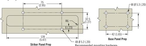
Recommended mounting hardware: M5 OR No.10 flat head screws
