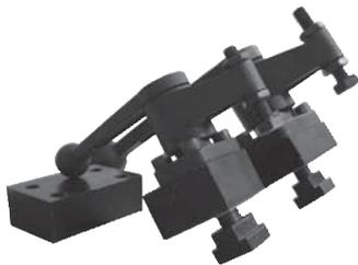
The height block assembly provides the user with a convenient method of setting the height of the Cam Swing Clamp when in operation. The act of locking the clamp onto the work piece also locks the block into position along the Tee Slot.
