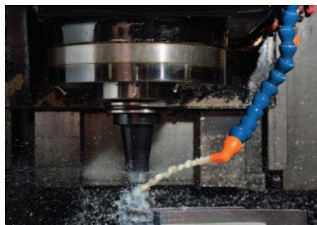
90° angle nozzle \varnothing 6
