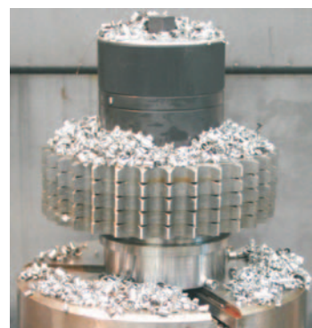
Clamp nut clamping sprockets during milling
