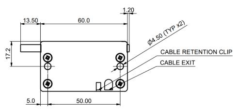
EXTENDED - MONITORING OUTPUT LOW BOLT TRAVEL IS ± 3.00mm
