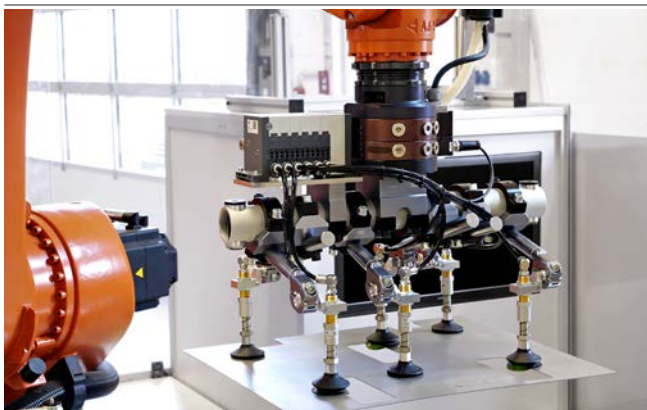
Clamping pieces SXT-CL for assembling a complete tooling for handling formed sheet metal parts
