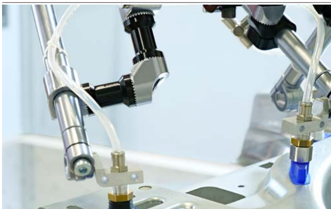
Connection (geared) SXT-CON-GB when handling a formed sheet metal part
