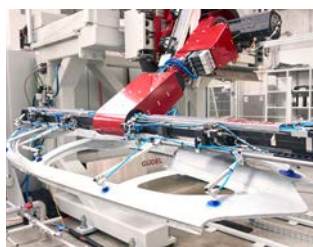
From Destacking Sheets to Unloading the Press
