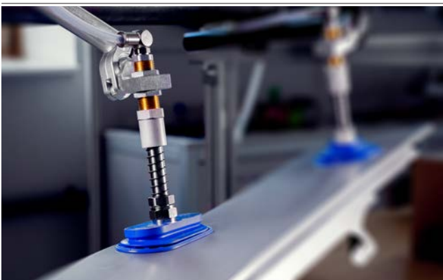
Holder for spring plunger HT-FST in combination with spring plunger FSTE-HDB for handling sheet metal parts
