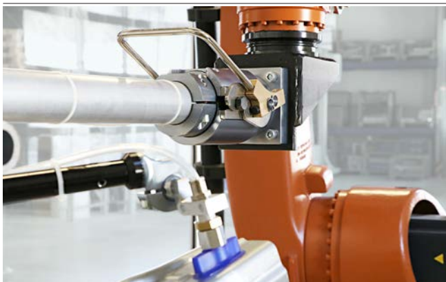
Quick-change robot bayonet SXT-QC-CON used for handling a formed sheet metal part
