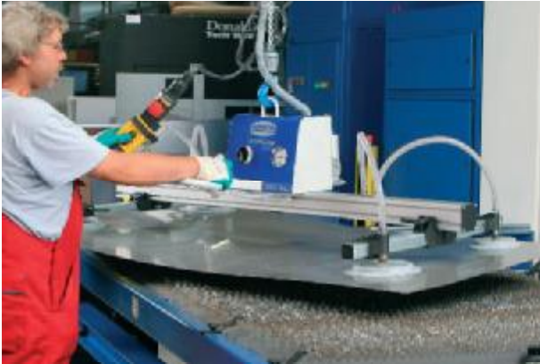
VacuMaster Basic, 250 kg Traglast, horizontal
