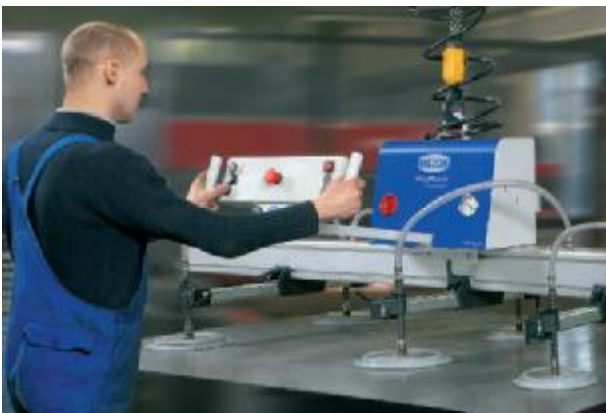
VacuMaster Comfort, 750 kg Traglast, horizontal
