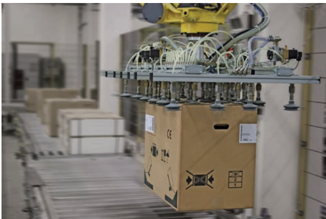
Customer-specific design of the vacuum suction spider SSP for handling various large cardboard boxes
