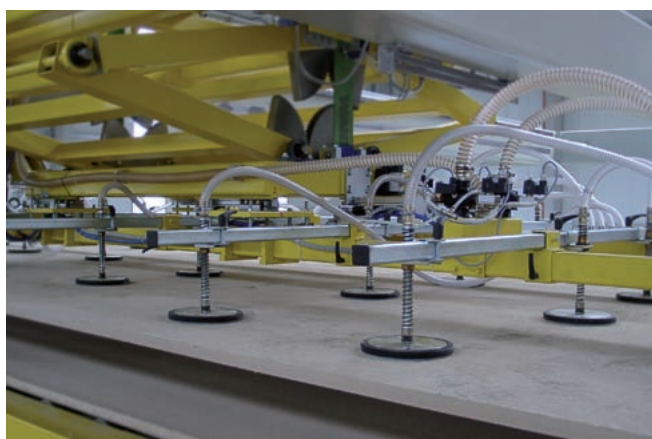
Vacuum suction spider SSP with suction plates
